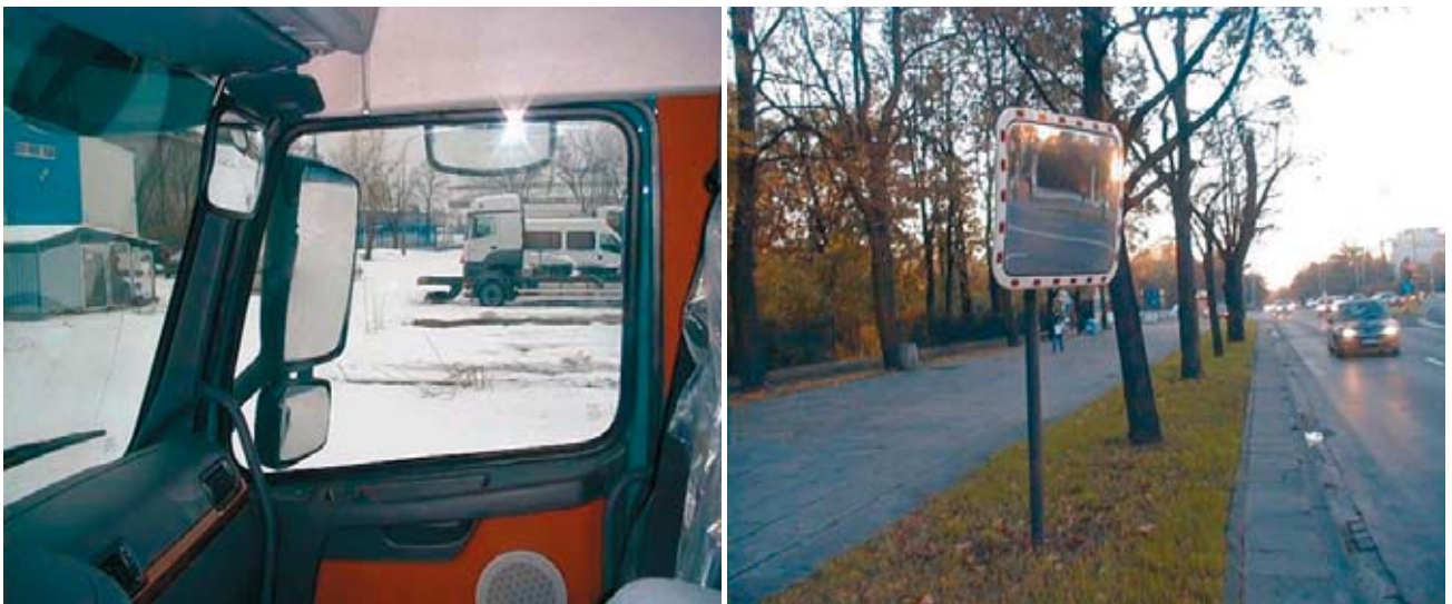
Fig. 12. Extra spherical mirror in vehicle cab and view of mirror placement on the road with the lack of visibility
